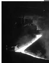
Slag Run-off from an Open Hearth Furnace
